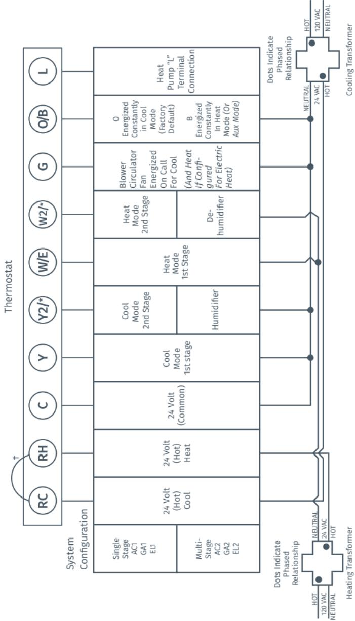
Two transformers systems (separate RC and RH wires), clip internal RC/RH jumper, located on back of thermostat.
