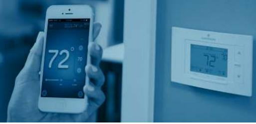
Pressing "Menu" at the thermostat allows you to change a series of settings to customize the thermostat for your specific system. Refer to the chart below for a complete listing of thermostat configurations and what they stand for. If you are installing the thermostat on the wall for the first time, we highly recommend that you download the Sensi app and follow the installation instructions.
